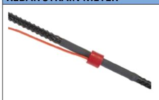
Model SIS - VWS-4000 series vibrating wire Rebar Strain Meters (often known as 'sister bars') are designed to be embedded in concrete to measure strains due to imposed loads in mass concrete. The location of installation defines whether it is a Rebar Strain meter or a Sister Bar.
